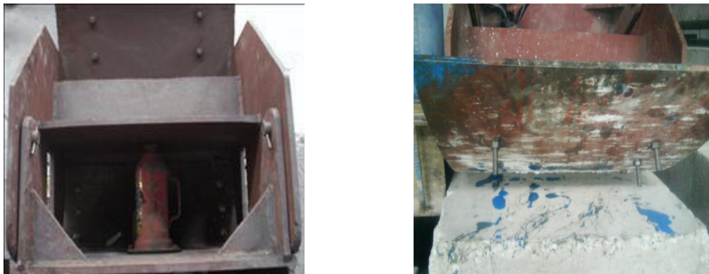
Fig. 5 Pre-stressing machine used for pre-stressing of sheets
