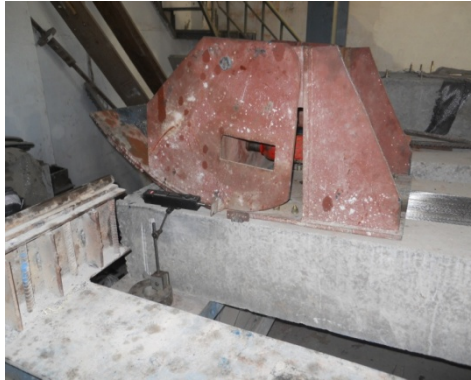
Fig. 7 LVDTs attached to both sides of the machine for measuring the elongation in fibre
