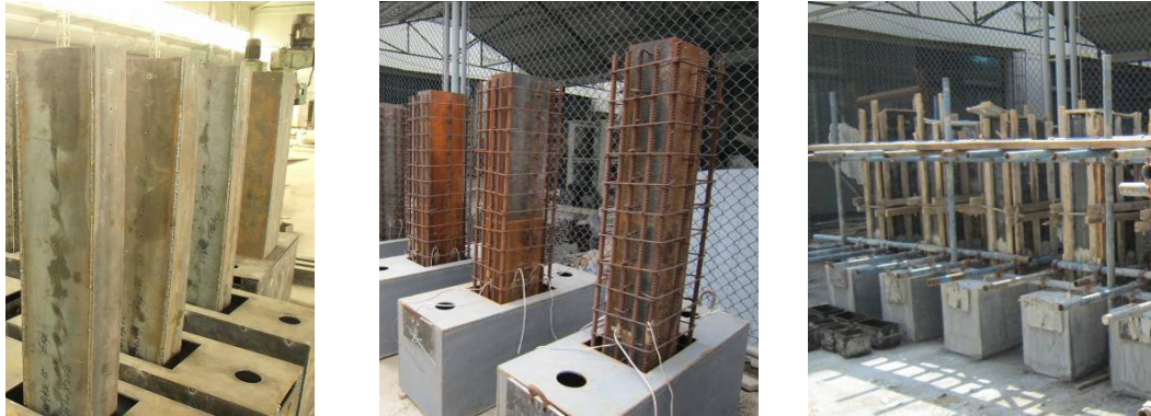
Fig. 2 Construction procedure of the test specimens
