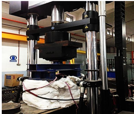
Fig. 4 Typical push out test setup for testing of shear connectors subjected to fire
