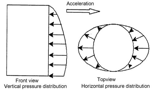
Fig. 2 Equivalent static loading
