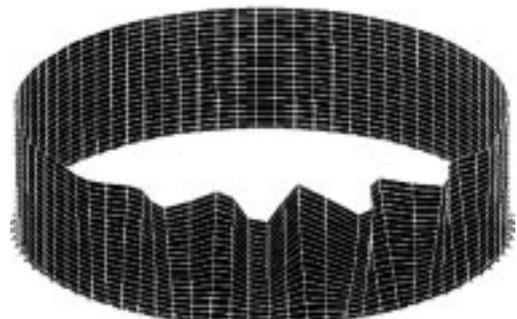
Fig. 6 FEM buckling mode
