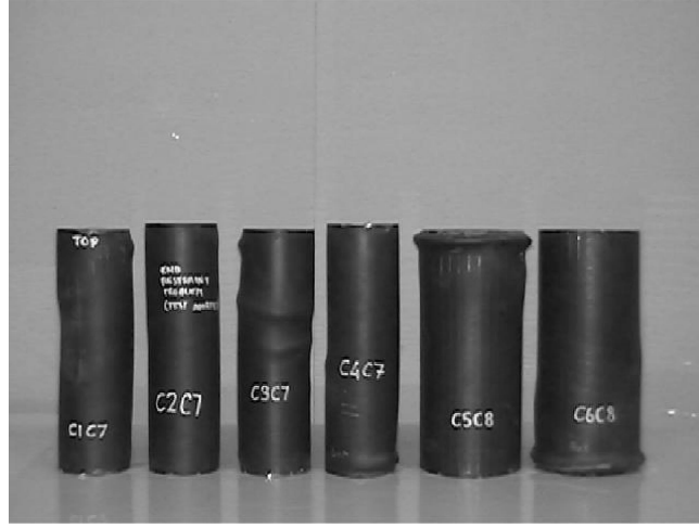
Fig. 7 CFDST specimens after testing
