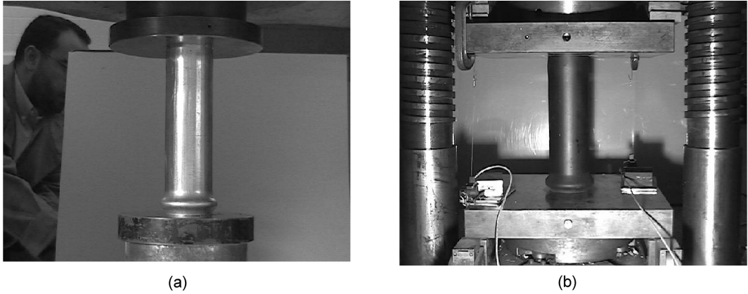
Fig. 3 Test set up (a) empty CHS stub columns in baldwin testing machine, (b) CFDST stub columns in amsler testing machine
