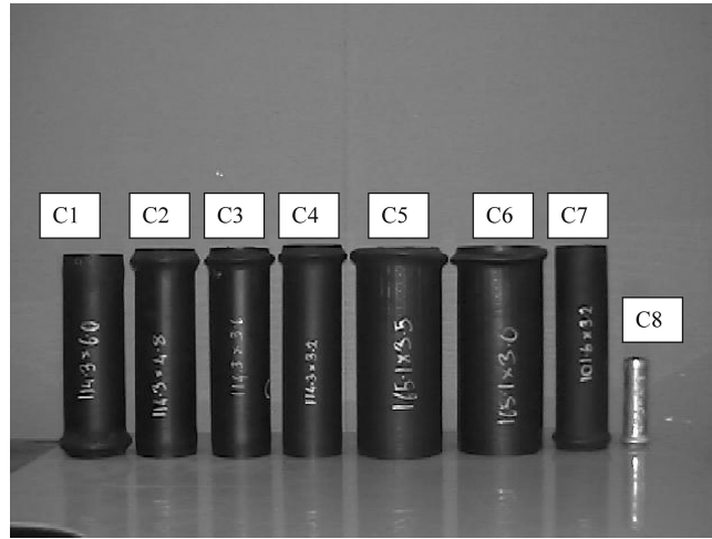
Fig. 4 Failure modes of empty CHS stub columns
