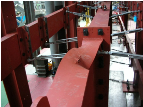
(c) Flange local buckling (TB-L/2)
