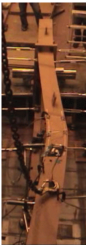
(b) Lateral torsional buckling (TB-250)
