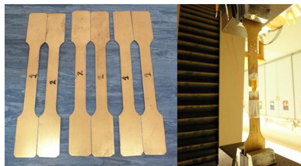
Fig. 5 Tensile coupon test: stress strain curve (left), specimens and failure (right)
