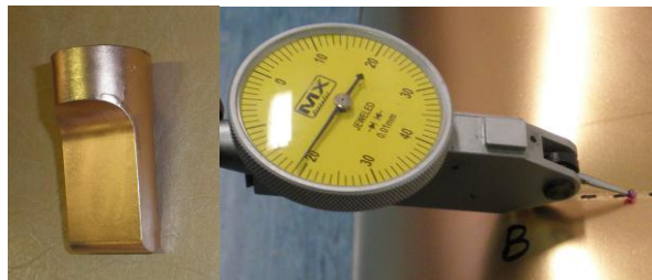
Fig. 4 Indenter (left), and gauge to measure the geometry of the dented area (right)
