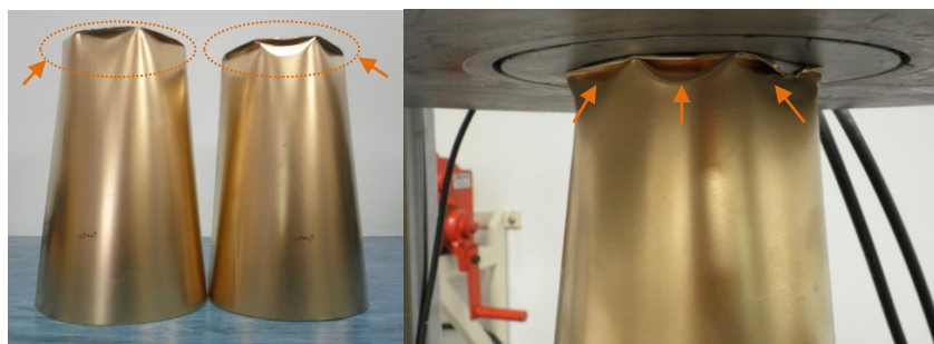
Fig. 7 Diamond mode of failure
