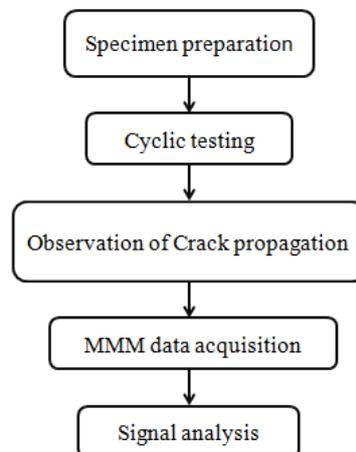
Fig. 6 Process flow of experimental method
