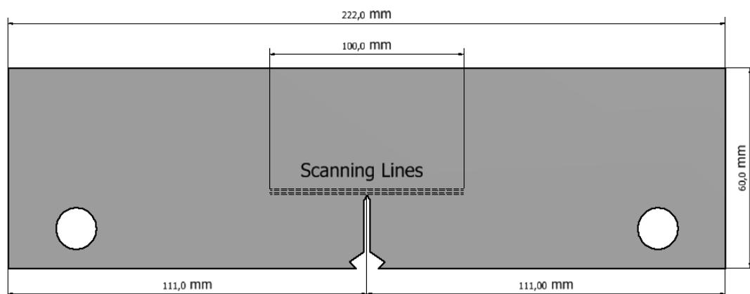
Fig. 2 Geometry dimensions of the notched fatigue specimen and the scanning line of the MMM signals
