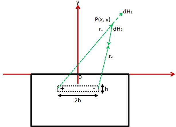
Fig. 1 Magnetic flux leakage field at a space point,  $P(x, y)$  based on Equivalent Plane Dipole model
