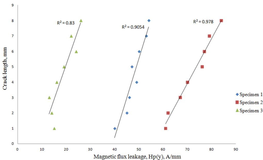
Fig. 12 Linear relation between the crack length and magnetic flux leakage from the MMM signals
