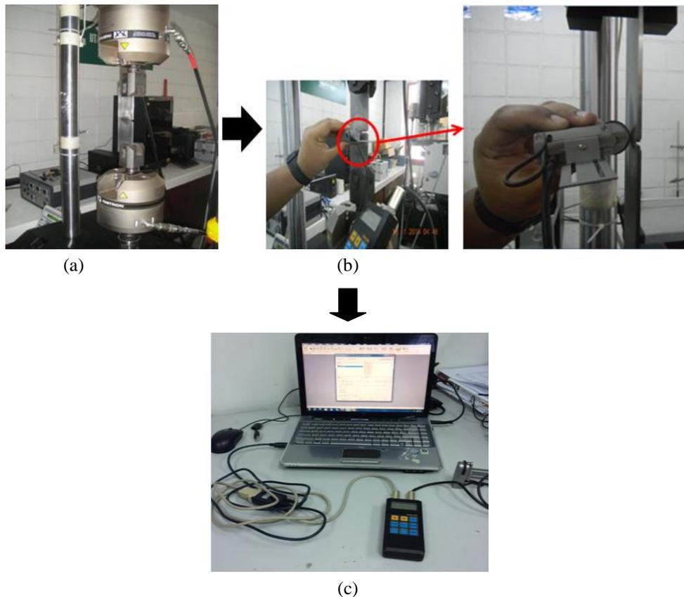
Fig. 3 Fatigue test set-up. (a) The servo-hydraulic machine with a specimen attached; (b) scanning process using MMM instrument; (c) MMM data collection through the computer using TSC-MMM-3.0 Software
