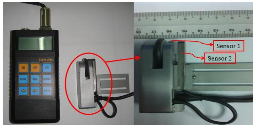
Fig. 4 The MMM instrument and scanning device
