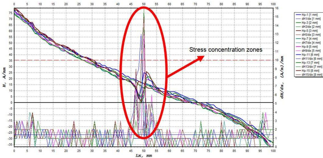
Fig. 9 The amplitude of SMLF signals,  $H_p(y)$  and  $dH/dx$  for specimen 3
