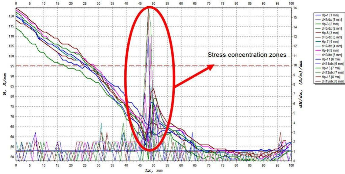
Fig. 8 The amplitude of SMLF signals,  $H_p(y)$  and  $dH/dx$  for specimen 2
