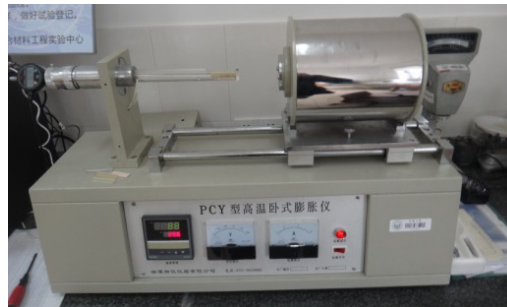
Fig. 5 PCY High temperature horizontal thermal expansion instrument
