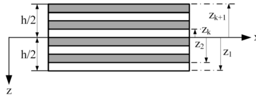
Fig. 2 Layer numbering used for a typical laminated beam
