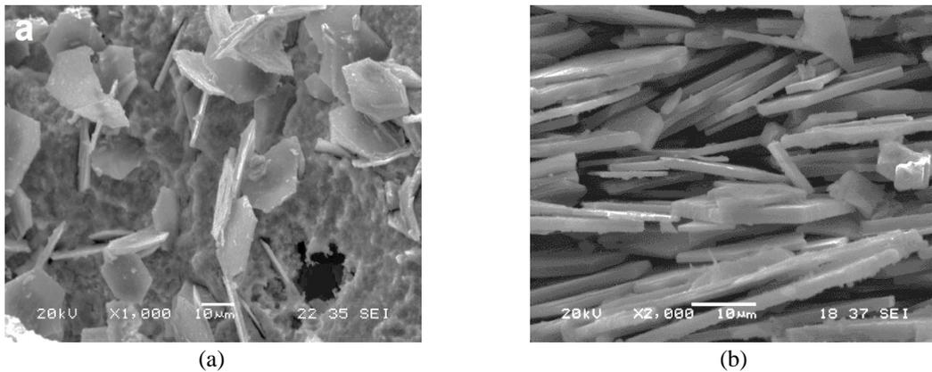
Fig. 5 SEM image of the deep etched: (a) as cast Al-B alloy before filtration; and (b)  $\text{AlB}_2/\text{Al}$  composite after filtration
