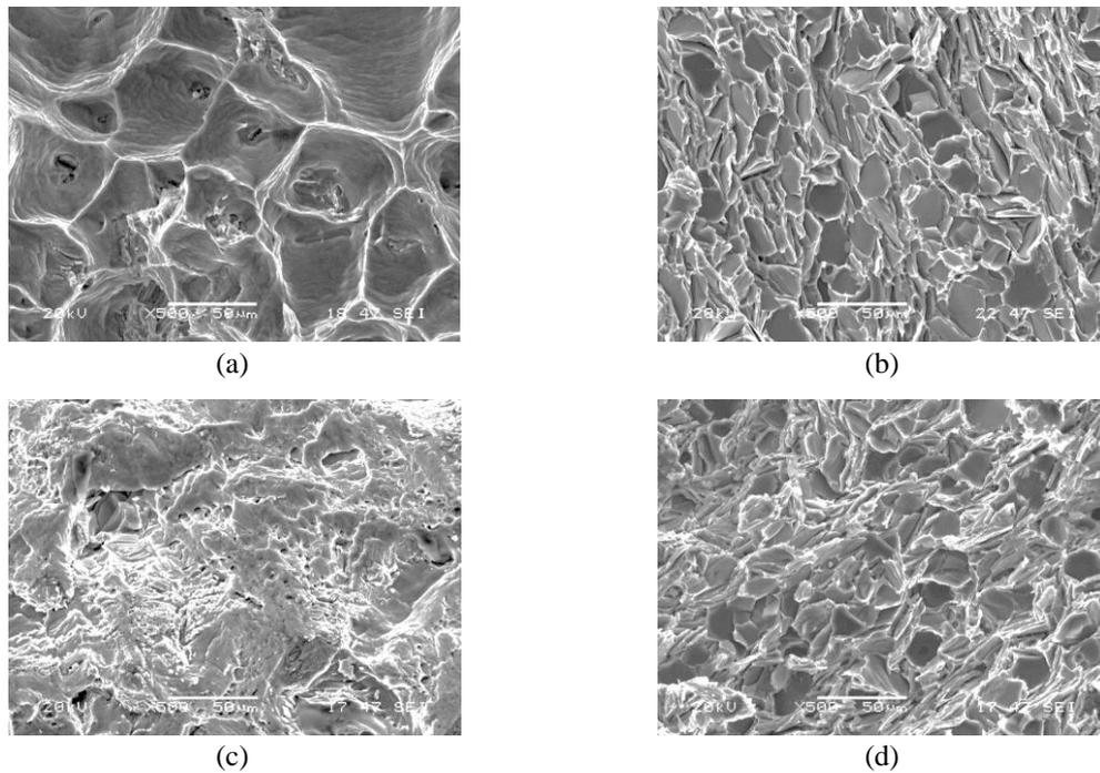
Fig. 8 SEM micrographs of the tensile fracture surfaces of; (a) commercially pure Al matrix; (b) AlB<sub>2</sub>/Al composite after filtration; (c) Al-4wt.% Cu matrix alloy; and (d) AlB<sub>2</sub>/Al-Cu composite after filtration
