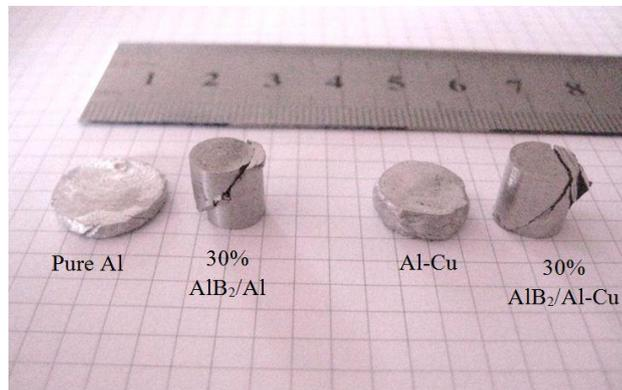
Fig. 7 Compressive strength test samples of the composites and their matrix materials
