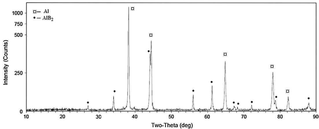
Fig. 4 The XRD spectra of the Al-B alloy
