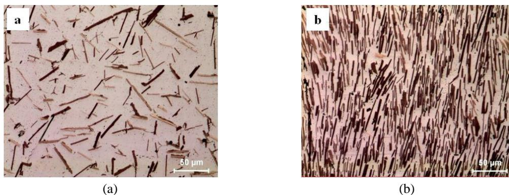
Fig. 3 Microstructure of (a) the as-cast master Al-B alloy; and (b) AlB<sub>2</sub>/Al composite material after filtration
