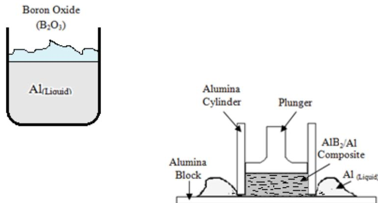
Fig. 2 The production scheme of the composite materials: (a) reaction melted aluminum with  $\text{B}_2\text{O}_3$  at 1300°C, structures; and (c) increase the  $\text{AlB}_2$  boride concentration by the filtration system at 700°C
