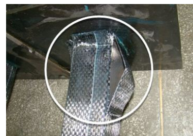
(j) Local buckling at end part (LN-20-3L)
