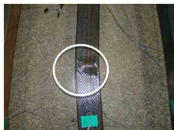
(i) Local buckling at mid-part (LN-20-1L)
