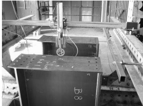
Fig. 5 Measuring the plastic deformations of the end-plate (specimen TB8)
