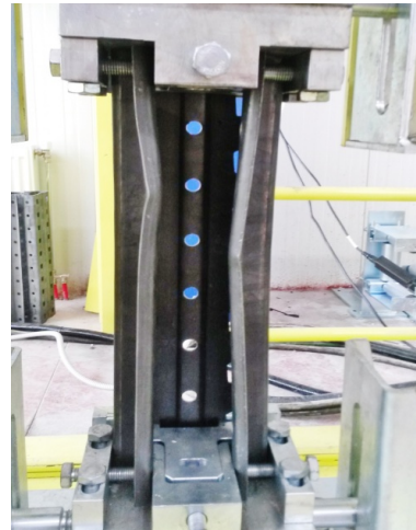
(b) Buckling occurs at the flanges
