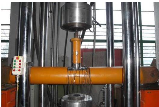
Fig. 2 View of test rig for CFCST T-joint specimen
