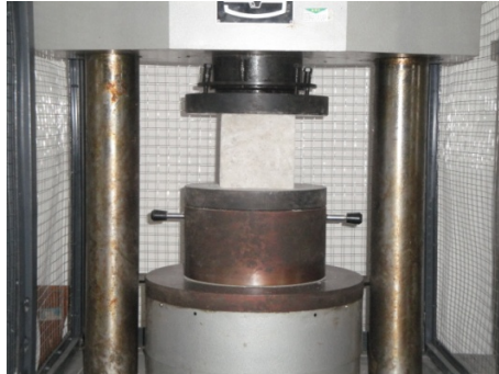
Fig. 2 Compressive test on measuring concrete strength
