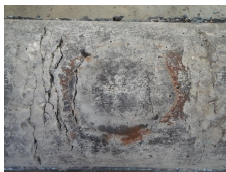
Fig. 10 Failure mode of core concrete
