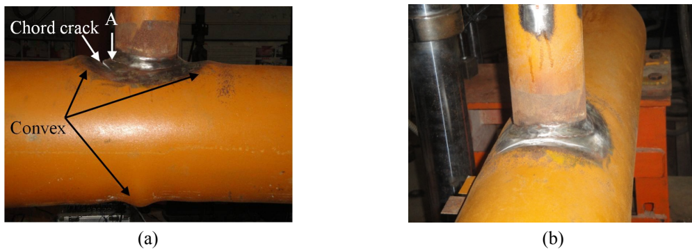
Fig. 6 Typical failure modes of specimen SP-A1
