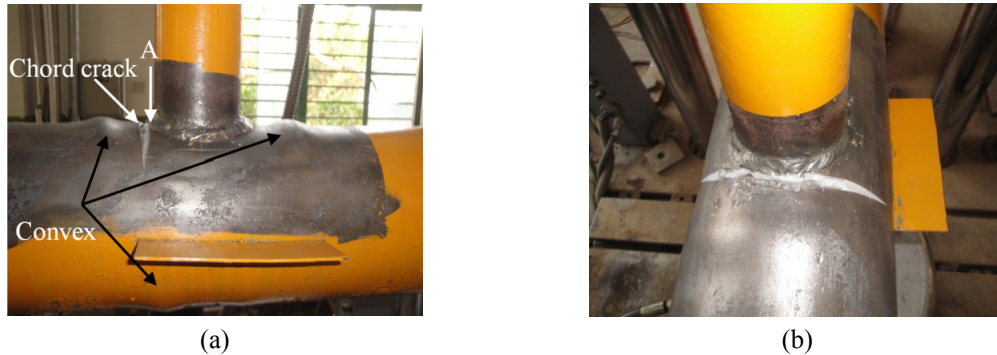
Fig. 9 Typical failure modes of specimen SP-B2
