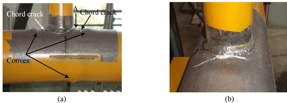
Fig. 8 Typical failure modes of specimen SP-B1
