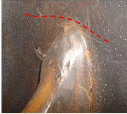
Fig. 7 Fatigue crack in s1
