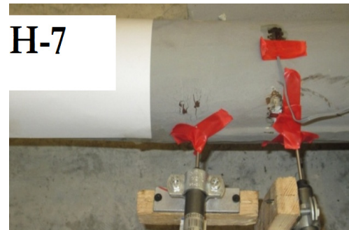
Fig. 16 Tearing of the steel tube in Test Unit H-7
