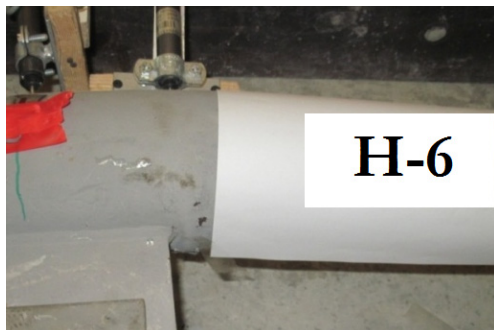
Fig. 15 Bulging of the steel tube under the gusset plate in Test Unit H-6
