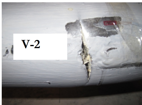
Fig. 13 Tearing of steel tube in Test V-2
