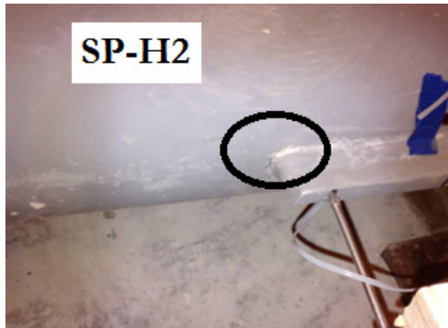
Fig. 5 Fracture of weld in Test SP-H2
