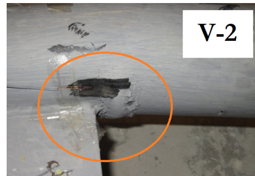
Fig. 12 Bulging of steel tube in Test V-2
