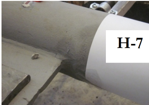
Fig. 17 Bulging of the steel tube under the gusset plate in Test Unit H-7
