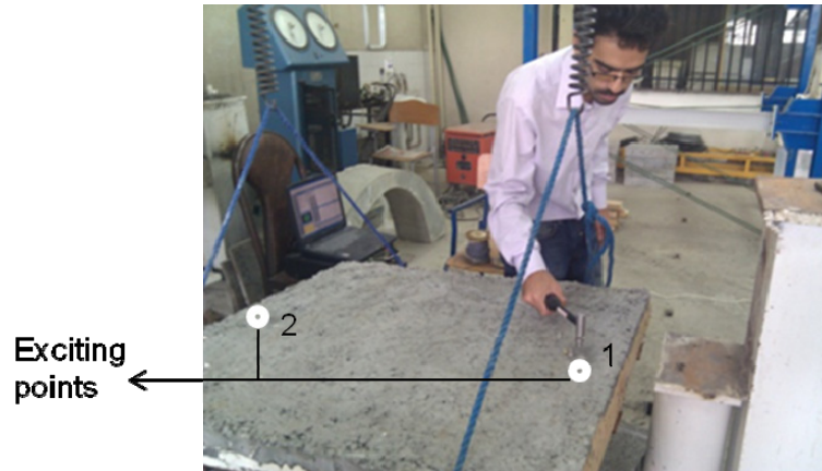
Fig. 7 Exciting the Exodermic deck by the impact hammer
