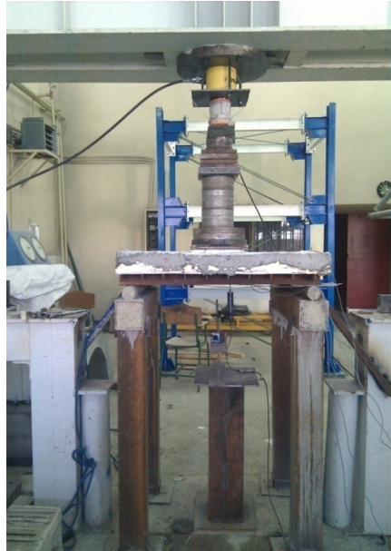
Fig. 13 Rigid parts used in order to provide stiffness between load-cell and the deck
