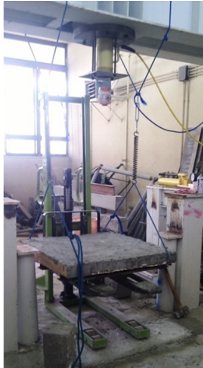
Fig. 6 An Exodermic deck suspended by two springs and ringed ropes
