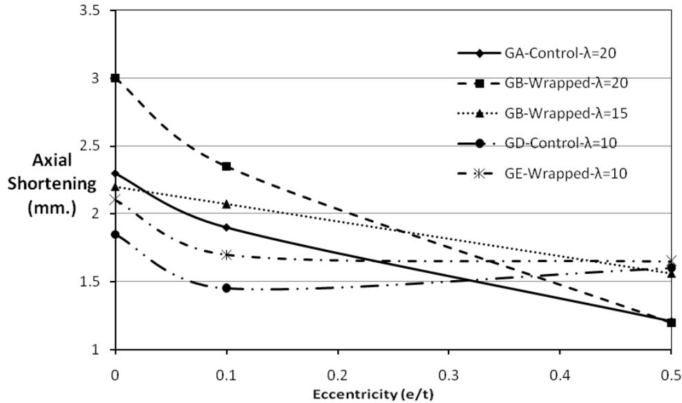
Fig. 5 Effect of confinement on axial shortening at failure
