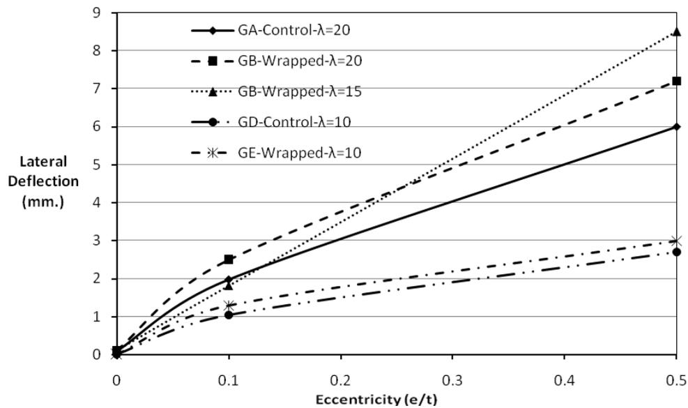
Fig. 6 Effect of confinement on lateral deflection at failure
