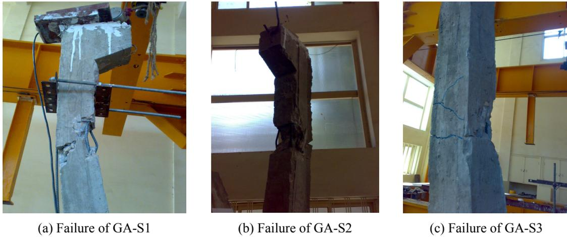
Fig. 7 Failure patterns of unwrapped slender columns
