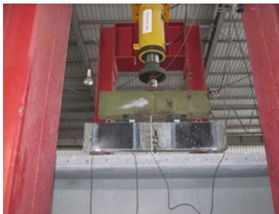
Fig. 4 Test set up for CFRP-strengthened RC deep beam
