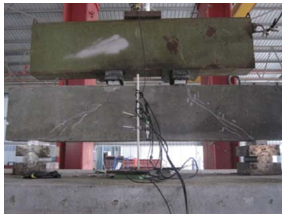
Fig. 3 Test set up for ordinary RC deep beam
