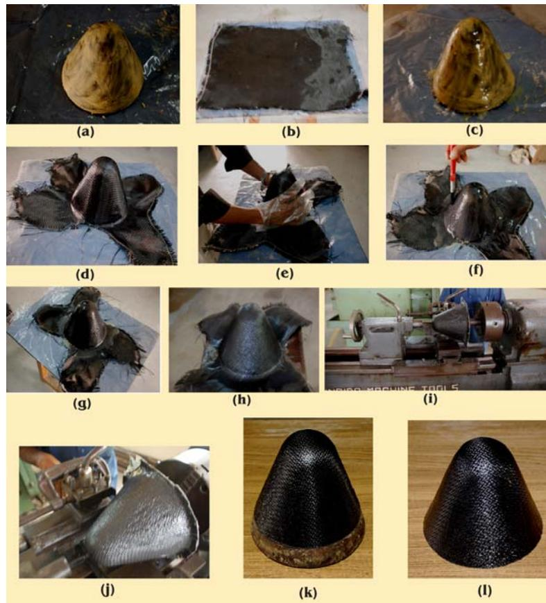
Fig. 4 CFRP shell-fabrication steps
