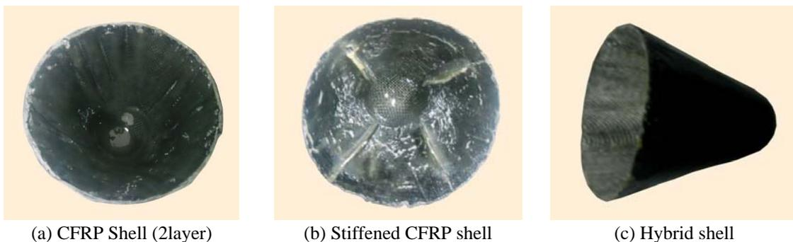
Fig. 8 Laminted / stiffened / hybrid shells
