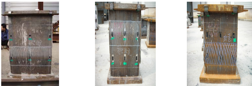
Fig. 5 Buckling patterns for Specimens 4, 5, and 6 (SS400)
