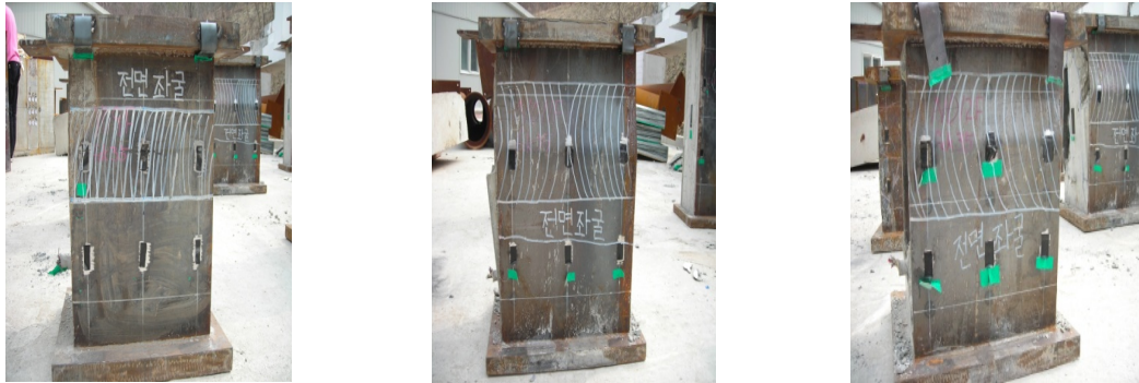
Fig. 4 Buckling patterns for Specimens 1, 2, and 3 (SM490)
