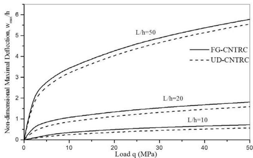
Fig. 5 Effects of plate length-to-thickness ratio  $L/h$  on the nonlinear bending behavior of CNTRC plates under transverse load  $q$  with  $V_{CN}^* = 0.11$  and  $T = 300$  K
