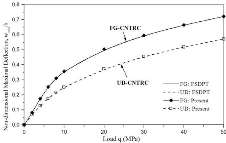
Fig. 2 Comparison of the central deflection for different theories versus load  $q$
