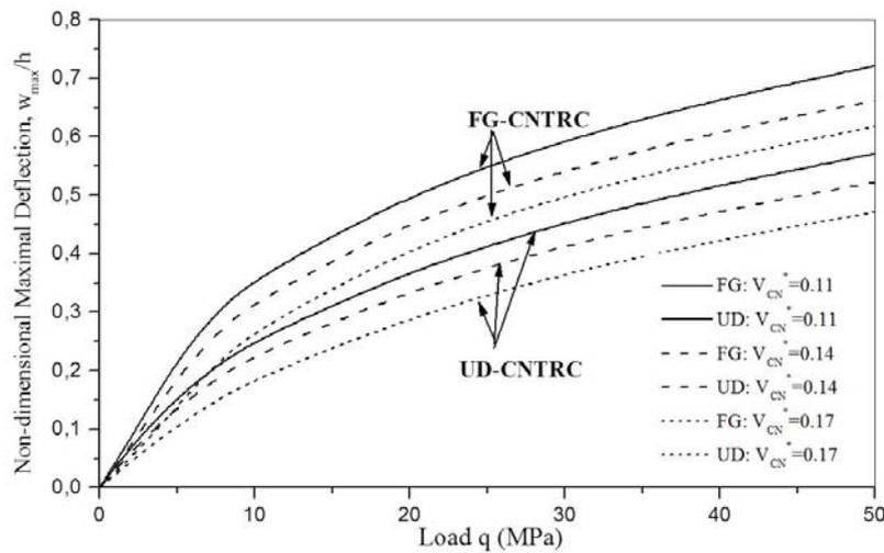
Fig. 3 Effects of nanotube volume fraction on the central deflection  $w_{max}$  of the CNTRC plate under uniform transverse load  $q$  and  $T = 300$  K
