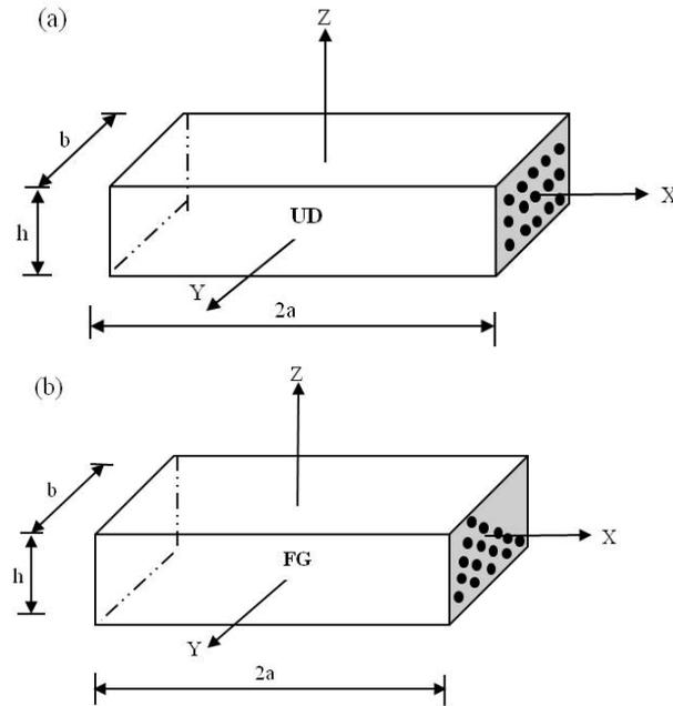
Fig. 1 Geometry of carbon nanotube-reinforced composites: (a) UD-CNTRC; and (b) FG-CNTRC
