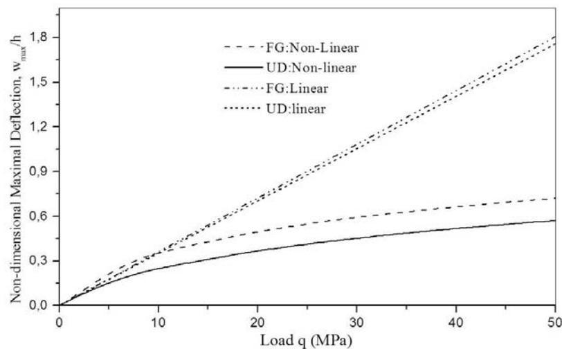
Fig. 4 Variation of the non-dimensional central deflection  $w_{\max}$  of the CNTRC plate versus transverse load  $q$  with  $V_{CN}^* = 0.11$  and  $T = 300$  K
