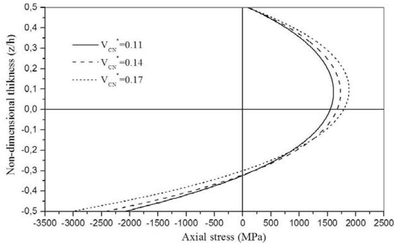
Fig. 6 Effects of nanotube volume fraction on the mid-span axial stress  $\sigma_x$  of the FG-CNTRC plate subjected to  $q = 50$  MPa and  $T = 300$  K with  $L/h = 10$
