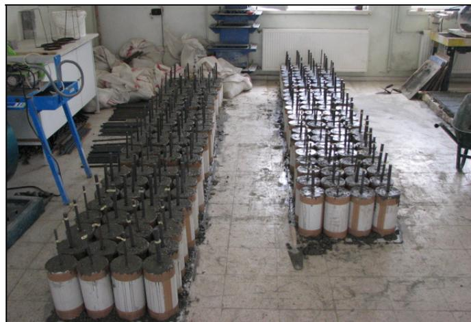
Fig. 2 Amount of lollipop shape test samples prepared for each concrete type
