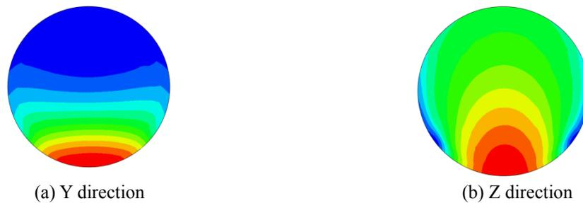
Fig. 4 Typical transverse stress distribution of confined concrete under a pure bending condition
