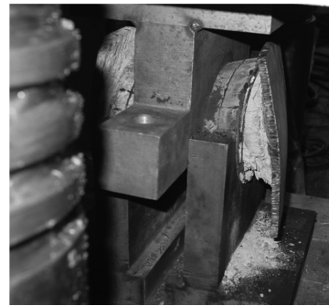
Fig. 11 Weld rupture of endplate
