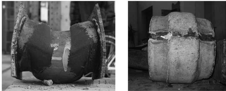
Fig. 3 Failure mode of specimens not sheared open
