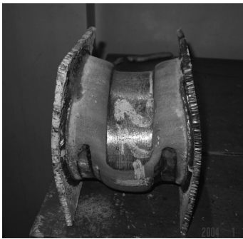
Fig. 10 Convex deformation of endplate
