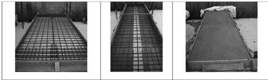
Fig. 5 Tested beams: slab with (on the left) and without (centre) profiled sheeting. Concrete cast of the slab (on the right)
