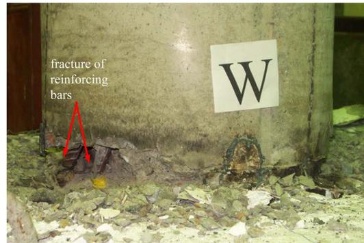
Fig. 10 Fracture of reinforcing bars in the plastic hinge zone at the bottom of composite pier (Specimen CC1)
