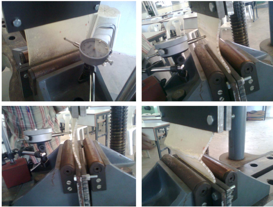
Fig. 3 Different stages in buckling test
