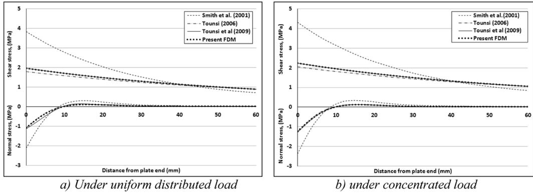
Fig. 3 Comparison of interfacial normal and shear stresses for CFRP-plated rectangular RC beam
