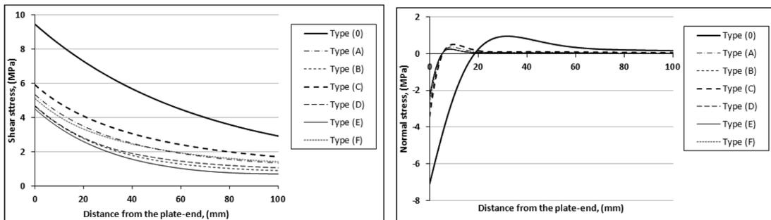
Fig. 6 Interfacial stress for various thickness taper of FRP plate.
