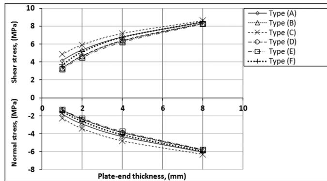
Fig. 8 Maximum interfacial stresses in terms of plate-end thickness for different taper profiles.
