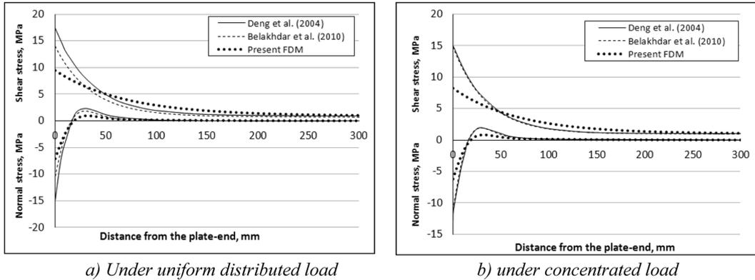
Fig. 4 Comparison of interfacial normal and shear stresses for CFRP-plated I-section steel beam
