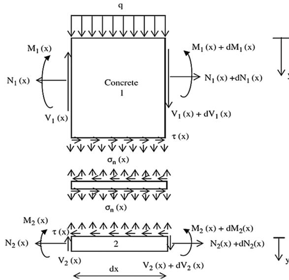
Fig. 2 Forces in infinitesimal element of a soffit - plated beam
