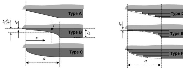
Fig. 5 Taper patterns of FRP plate.
