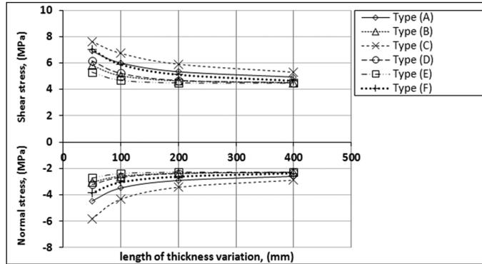
Fig. 7 Maximum interfacial stresses in terms of taper length for different taper profiles.
