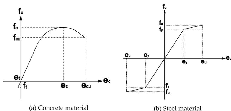
Fig. 12 Stress-strain relationship of the materials
