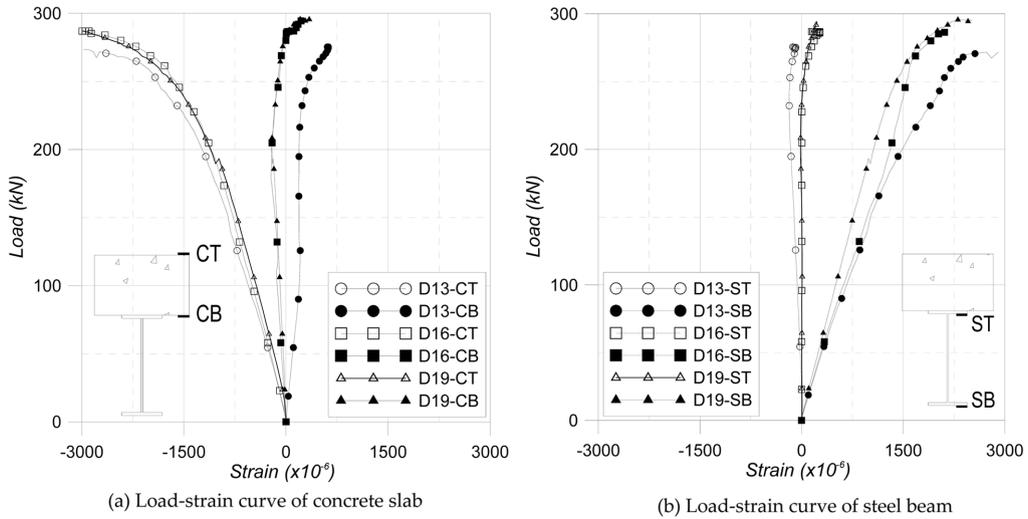
Fig. 8 Load-strain relationships of the composite beams
