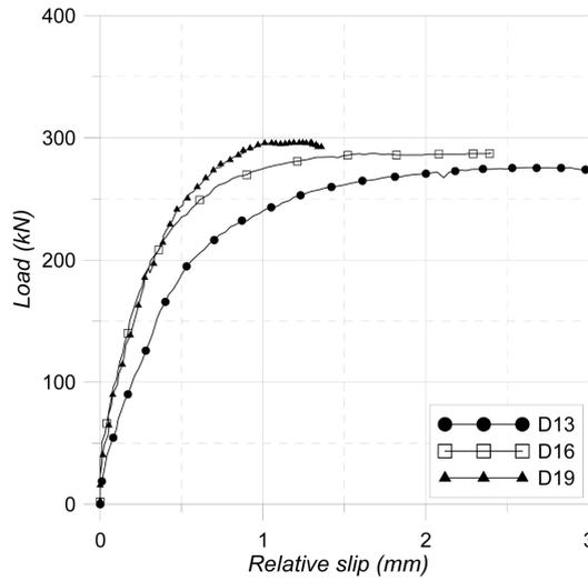
Fig. 10 Load-relative slip relationships at support of composite specimens
