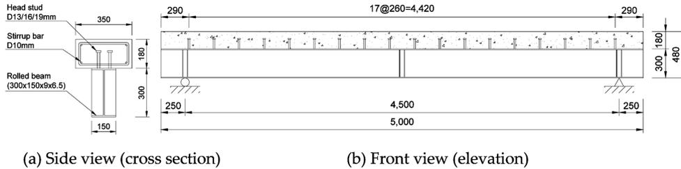
Fig. 3 Composite beam specimen
