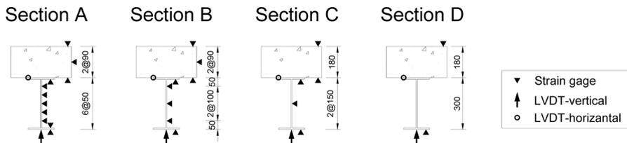
(b) Location of instrumentation at measuring section
