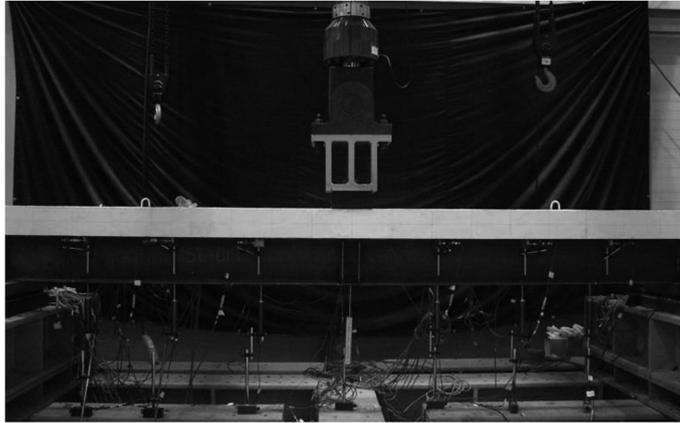
Fig. 5 Load test specimen and test set-up
