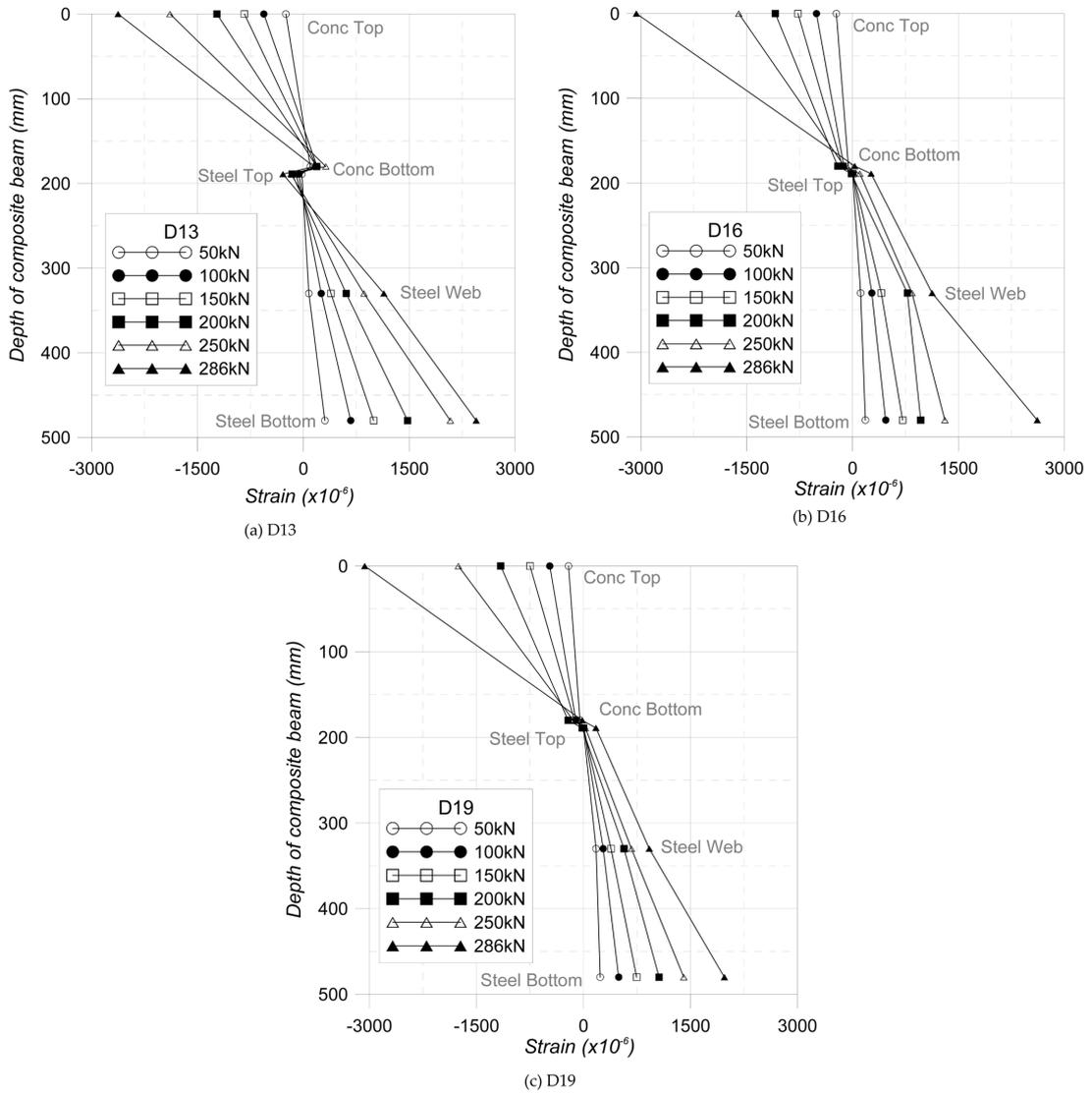
Fig. 9 Load-strain distribution at central section of the composite beams
