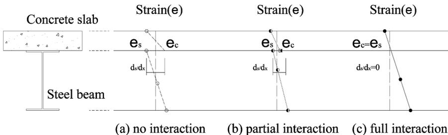
Fig. 2 Interaction behavior of composite beam
