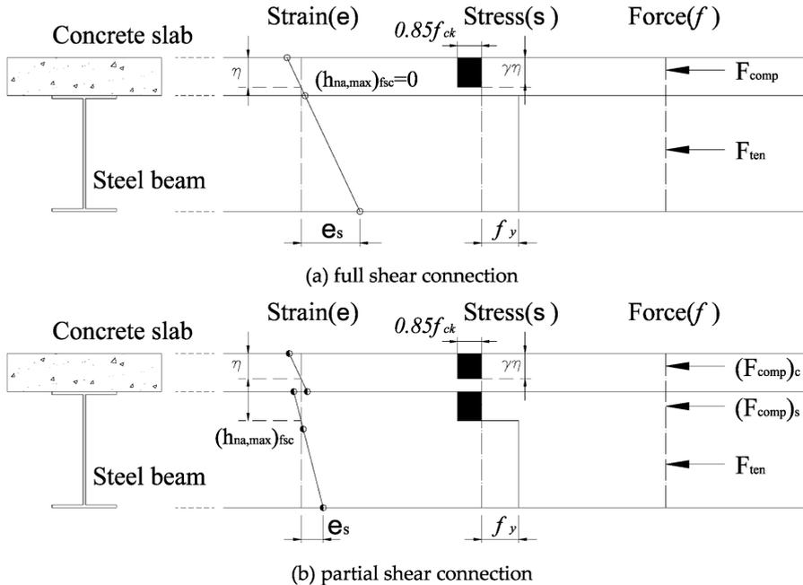
Fig. 1 Degree of shear connection in composite section
