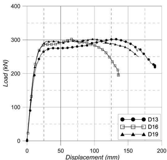
Fig. 7 Load-displacement relationships at center of composite specimens
