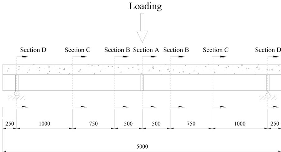
(a) Loading and measuring section
