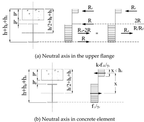
Fig. 11 Plastic moment of composite beam
