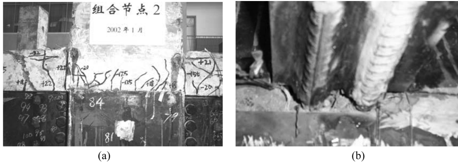
Fig. 10 Specimen GJD02 after test: (a) concrete cracks, (b) failure of the X-shaped bar
