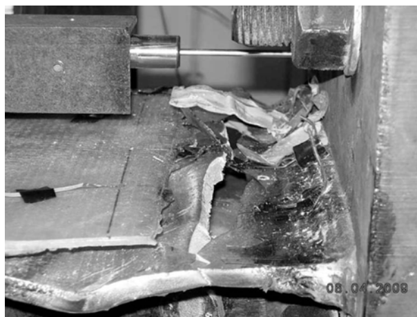
Fig. 16 Fracture of heat effected zone of specimen G3
