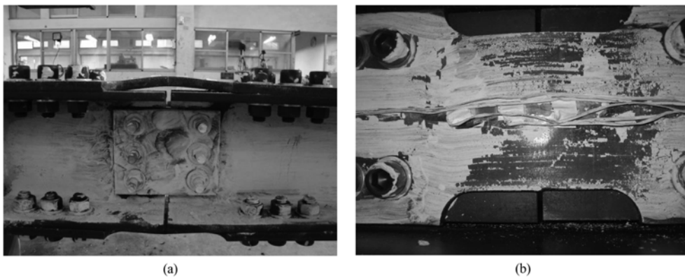
Fig. 7 Failure modes of the energy dissipation plates: (a) buckling under compression; (b) yielding under tension
