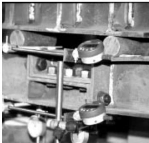
Fig. 7 Particular of joint with transducers
