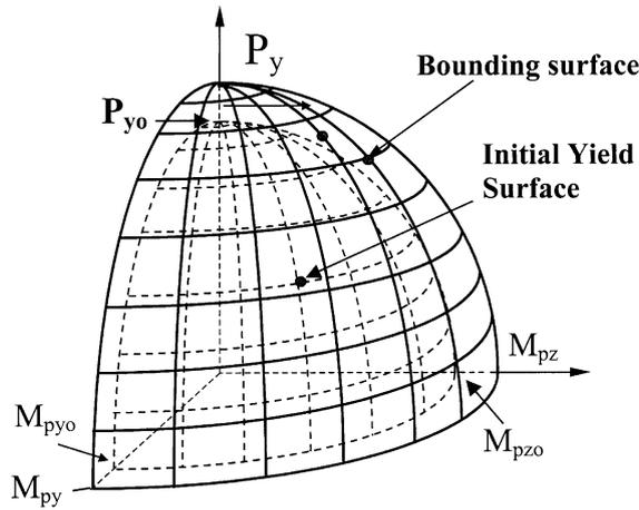
Fig. 3 Two surface plasticity model
