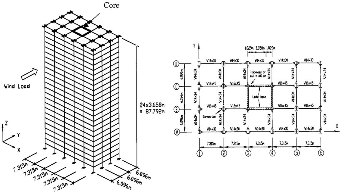
Fig. 7 Multistorey frame with “strong” core
