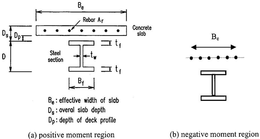
Fig. 4 Composite beam sections
