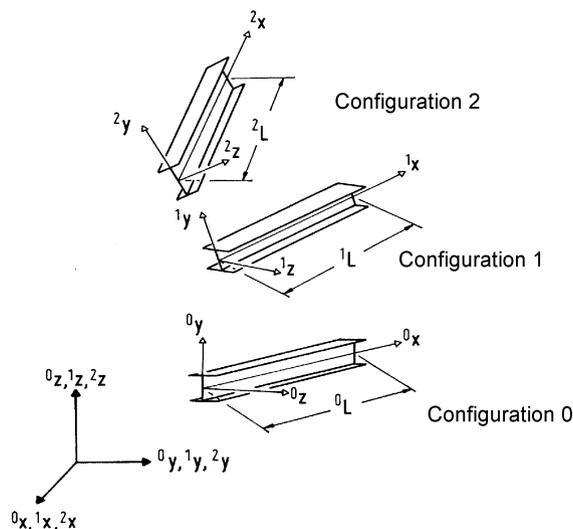
Fig. 2 Motion of beam column element based on update Lagrangian formulation
