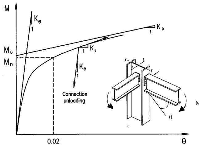
Fig. 6 Four-parameter power mode for connections
