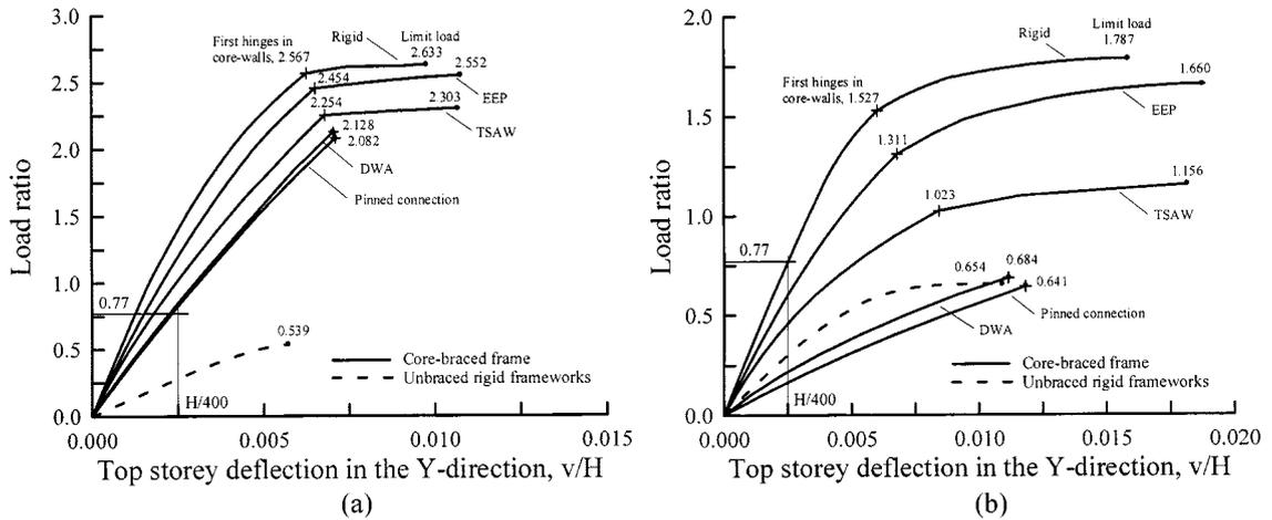
Fig. 9 Nonlinear inelastic analysis of core-braced frames (a) frame with "strong" core walls, (b) frame with "weak" core walls
