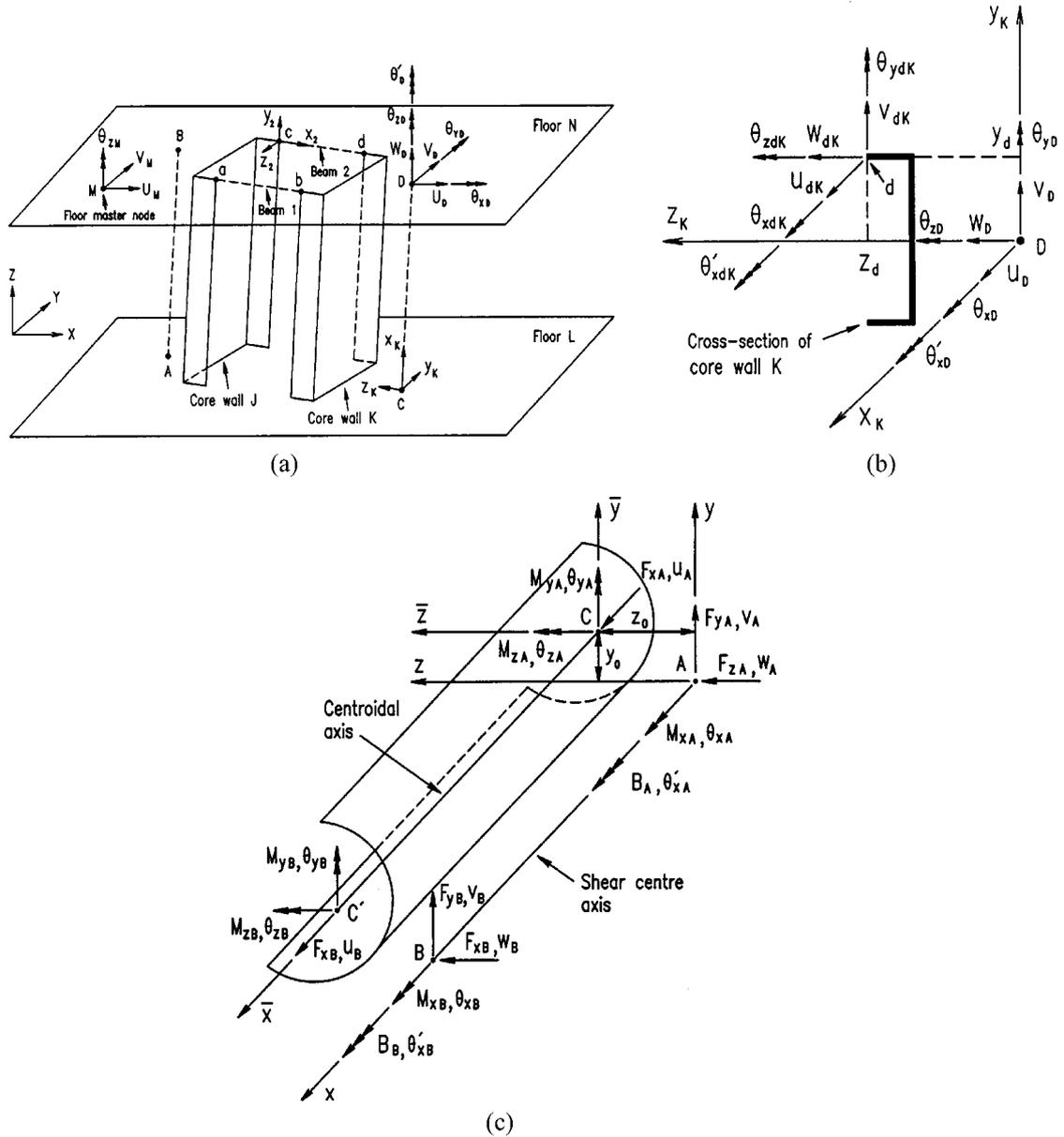
Fig. 5 (a) A building core wall between two floors, (b) Deformations of a thin-walled cross section, (c) A generic model for a thin-walled beam-column member
