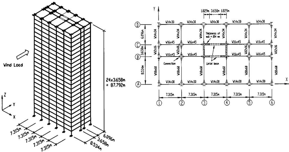
Fig. 8 Multistorey frame with “weak” core
