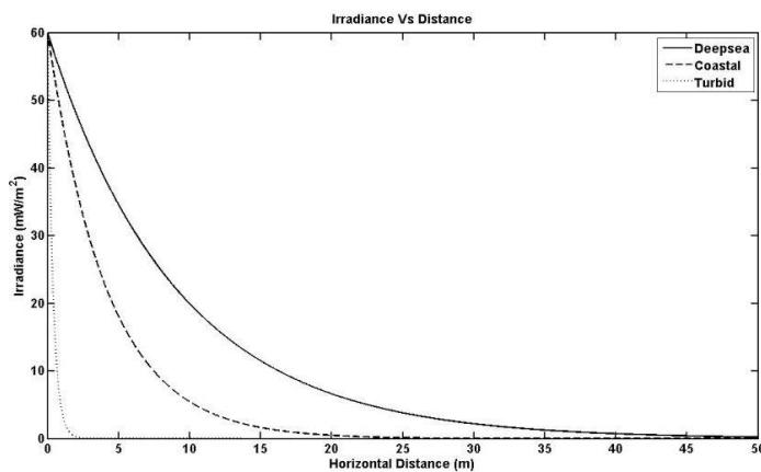
Fig. 4 Link distances in various ocean waters for 300 mW transmitter power
