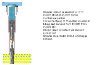
Fig. 3-6 Secondary Cement and Mechanical Barrier in Casing Section & Cement in Tubing
