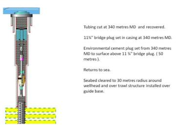
Fig. 3-8 Bridge Plug in Casing and Environmental Cement Plug Set
