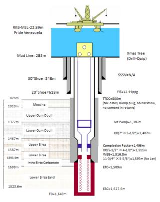
Fig. 3-2 Scheme of Producer Well (W-1)
