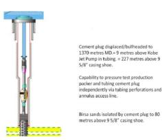
Fig. 3-5 Primary Cement Plug in Reservoir and Mechanical Barrier in Casing Section
