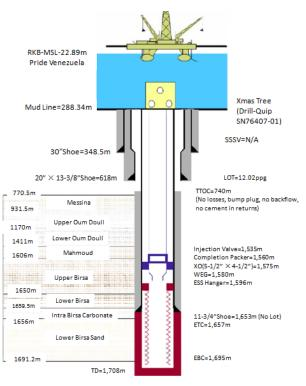
Fig. 3-3 Scheme of Injector Well (W-2)
