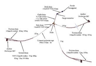
Fig. 2-2 The Layout of FPSO Mooring System
