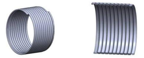
Fig. 1 Typical geometry of the interlocked pressure armor
