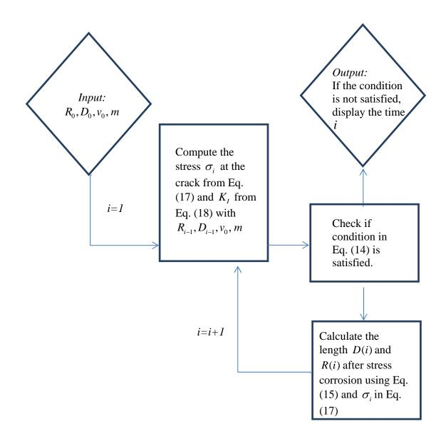
Fig. 2 Iterative algorithm for evaluation the time of service
