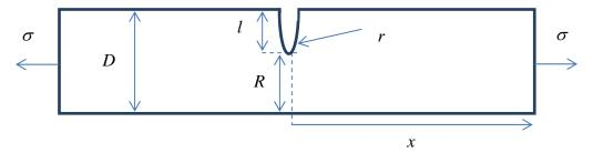
Fig. 1 Cracked bar under a tensile stress
