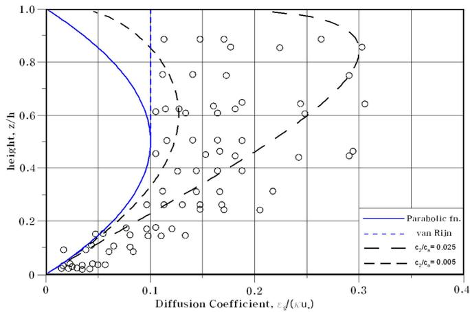
Fig. 5 Composition of computed and measured sediment diffusion coefficient ( $w_f / (\kappa U_*^2) = 0.833$ )
