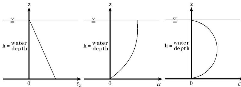
Fig. 1 Vertical distribution of shear stress, velocity, and fluid diffusion coefficient in water column
