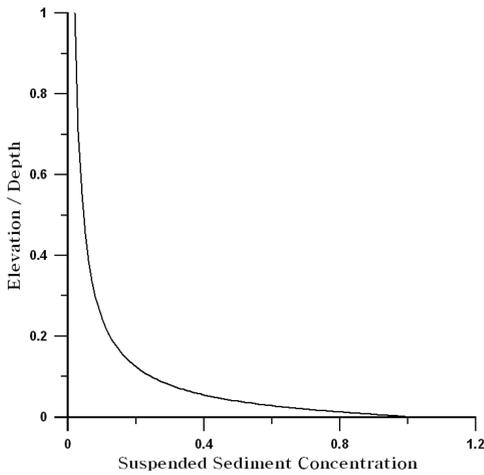
Fig. 2 Typical concentration profile of coarse sediment
