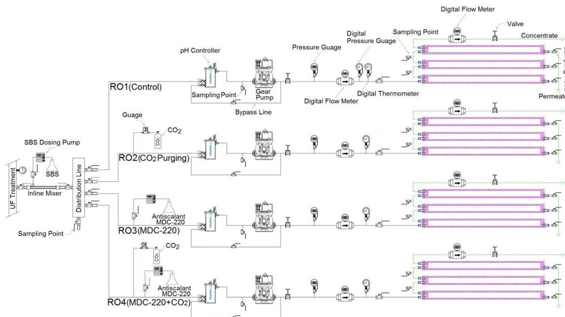
Fig. 1 Schematic diagram of the RO modules
