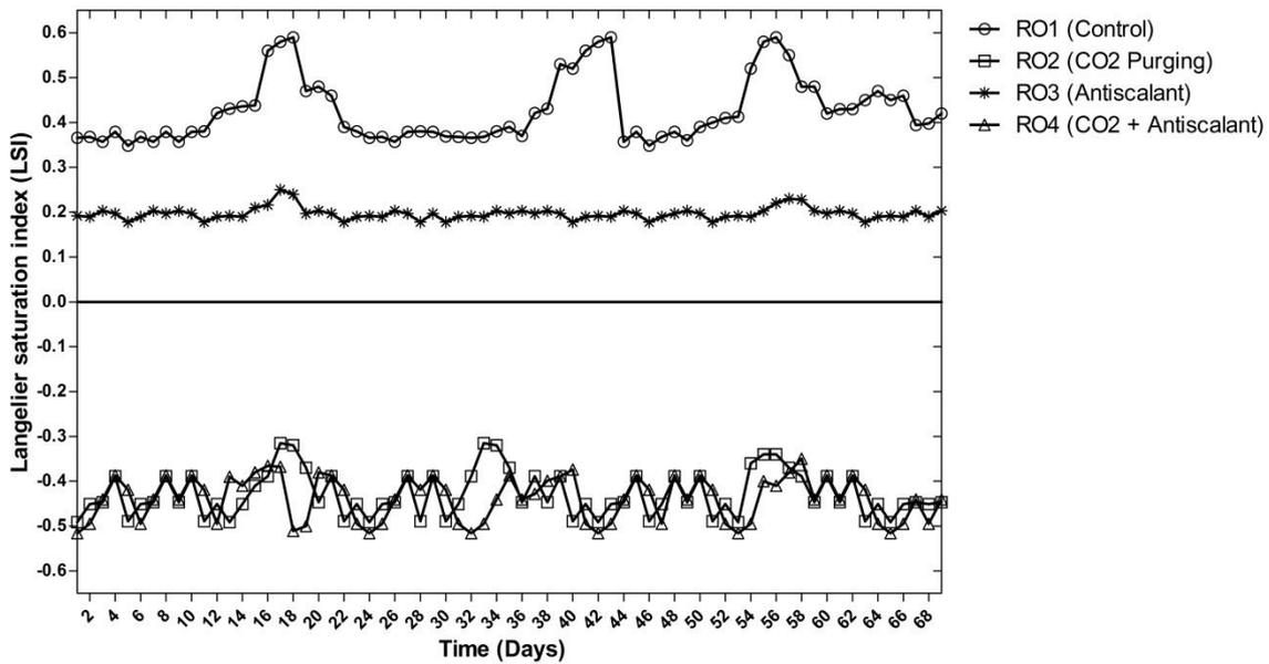
Fig. 3 Comparison between LSI data of all RO modules
