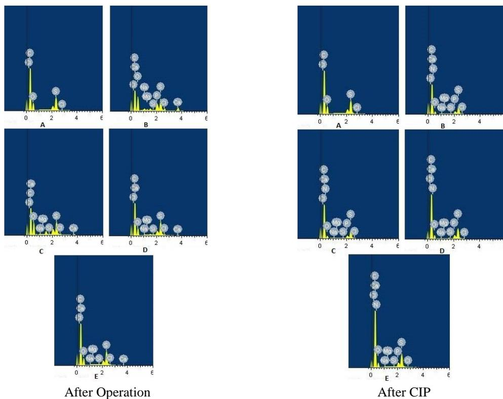
Fig. 7 EDS spectra of virgin (A), control (B), CO<sub>2</sub> injected (C), Antiscalant dosed (D), Antiscalant dosed + CO<sub>2</sub> injected (E) membrane
