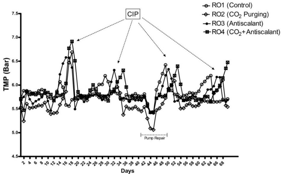
Fig. 2 Comparison of RO modules, change in TMP
