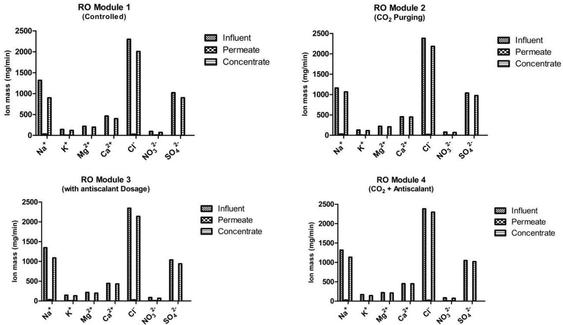
Fig. 4 Ion mass balance of RO modules
