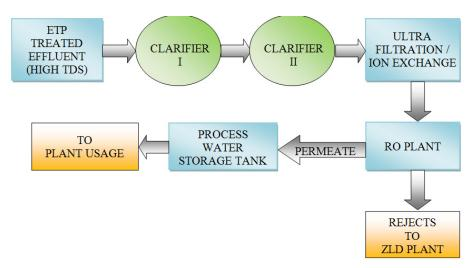
Fig. 6 Block diagram (modified) for the RO plant in copper industry
