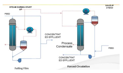
Fig. 8 Flow diagram (modified) showing "Evaporation with Mechanical Vapor Recompression (MVR)"
