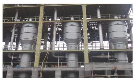
Fig. 5 Site photo showing "Multi Effect Evaporator using TVR"
