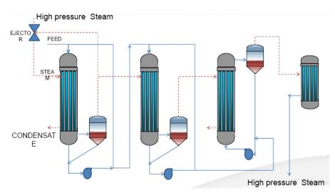
Fig. 4 Flow diagram showing "Multi Effect Evaporator using Thermal Vapor Recompression (TVR)"; Thermal Vapour Recompression, TVR
