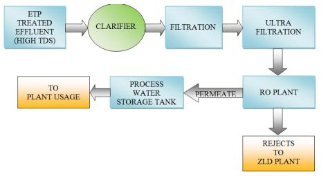
Fig. 2 Block diagram for UF/RO plant in copper industry
