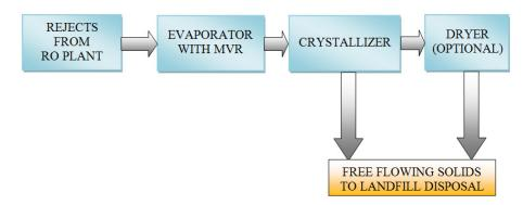
Fig. 7 Block diagram (modified) for Zero Liquid Discharge (ZLD) in copper industry
