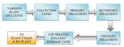
Fig. 1 Block diagram for effluent treatment plants in copper industry
