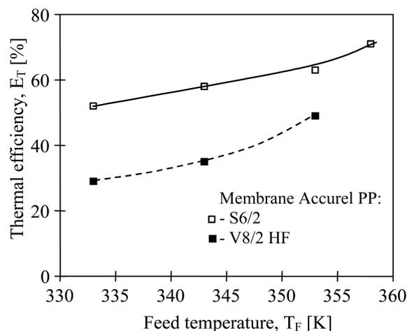
Fig. 5 The influence of feed temperature and membrane wall thickness on the thermal efficiency in MD process. Wall thickness: Accurel PP S6/2 – 400  $\mu\text{m}$ , Accurel PP V8/2 HF – 1550  $\mu\text{m}$ . Data for Accurel PP S6/2 were taken from (Gryta 2006)
