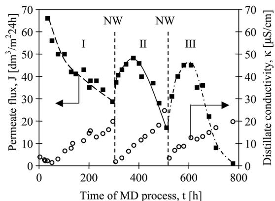
Fig. 10 Changes on the permeate flux and the electrical conductivity of distillate during the concentration of geothermal water by MD process (series I-III). Module MK2. NW – exchange of retentate into a new portion of fresh geothermal water
