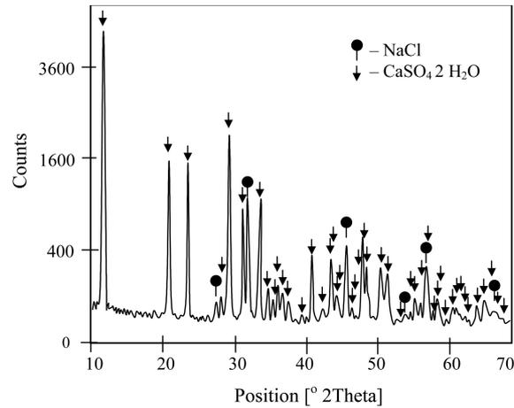
Fig. 13 The results of XRD analysis of deposit taken from the membrane surface (Fig. 11)
