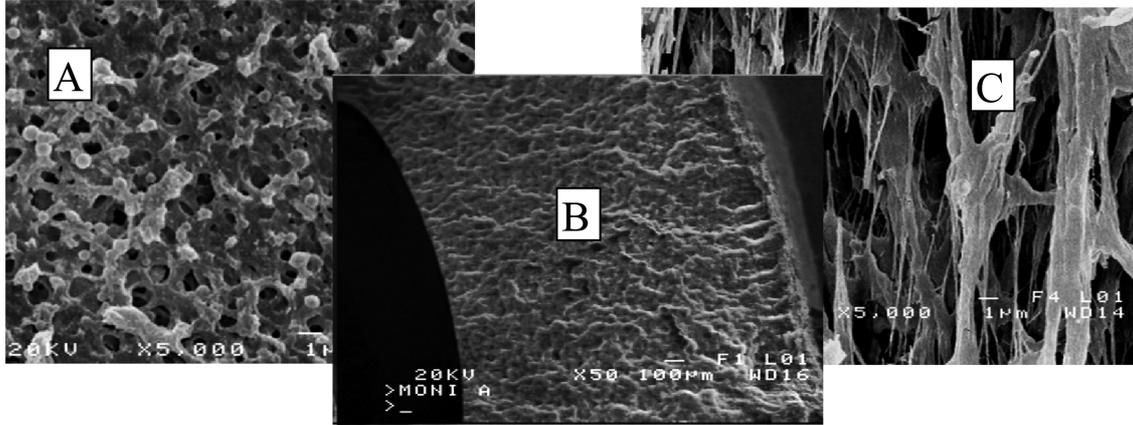
Fig. 2 SEM images of polypropylene capillary Accurel PP V8/2 HF membrane: A – internal surface, B – cross-section, C – external surface
