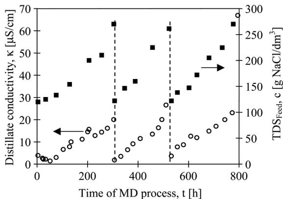
Fig. 9 Changes in the feed concentration (TDS-  $\text{g NaCl}/\text{dm}^3$ ) and the electrical conductivity of distillate during the concentration of geothermal water by MD process. Module MK2
