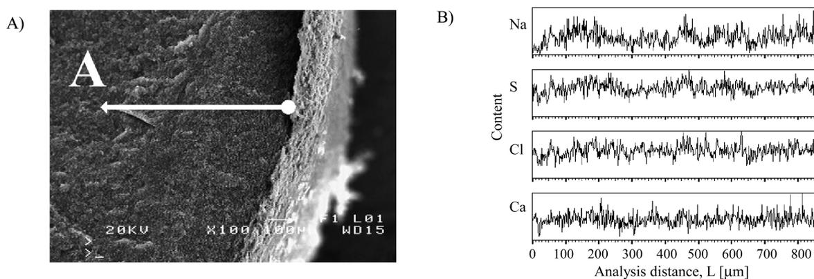
Fig. 8 The results of SEM investigations. A) cross-section of membrane taken from MK1 module after 800 h of geothermal water desalination, B) SEM-EDS line analysis (direction A from Fig. 8A)
