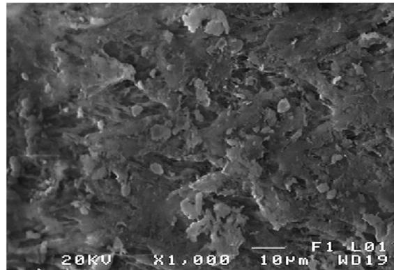
Fig. 7 SEM images of silicate deposit formed on the external surface of Accurel PP V8/2 HF membrane after 800 h of geothermal water desalination
