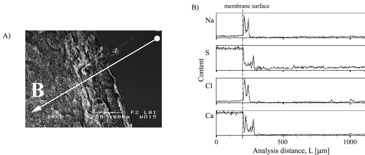
Fig. 14 The results of SEM investigations. A) cross-section of membrane, containing a deposit layer, taken from MK2 module after 800 h of geothermal water concentration. B) SEM-EDS line analysis (direction B from Fig. 14A)
