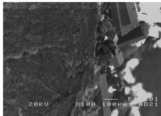
Fig. 12 SEM images of the cross-section of Accurel PP V8/2 HF membrane covered by deposit. Module MK2
