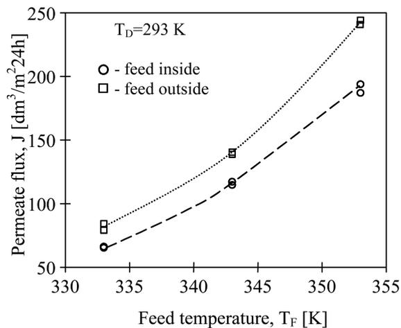
Fig. 3 The influence of feed temperature and flow direction on the permeate flux. Module MK1. Feed – distilled water. Feed inside – feed enters bore of the capillary. Feed outside – feed flowed on the shell side
