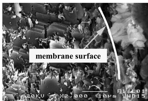
Fig. 15 SEM images of the membrane cross-section with pores destroyed by formed  $\text{CaSO}_4 \cdot \text{H}_2\text{O}$  crystallites
