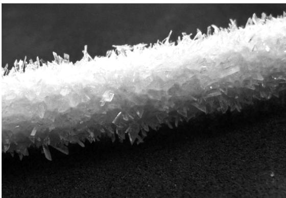
Fig. 11 SEM image of crystallite deposit on the external surface of Accurel PP V8/2 HF membrane
