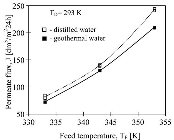
Fig. 4 The influence of feed temperature and salt concentration on the permeate flux. Module MK1. Distilled water (0 g NaCl/ $\text{dm}^3$ ), geothermal water (120 g NaCl/ $\text{dm}^3$ )
