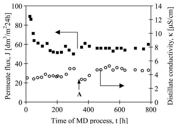
Fig. 6 Changes in the permeate flux and the electrical conductivity of distillate during the long-term geothermal water desalination. Module MK1. Mode: constant feed concentration (120 g NaCl/dm<sup>3</sup>). Point A – distillate side refilled with new distilled water (3 µS/cm)
