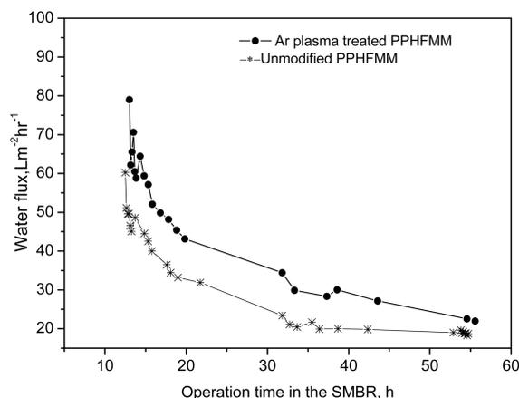
Fig. 3 Change of flux with operation time in the SMBR
