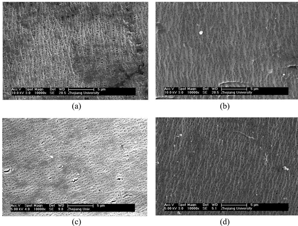
Fig. 1 FE-SEM images of the PPHFMMs. (a) Nascent PPHFMM; (c) The surface modified PPHFMM after 1 min Ar plasma treatment; (b) Nascent PPHFMM used in the SMBR; (d) Ar plasma treated PPHFMM used in the SMBR, respectively
