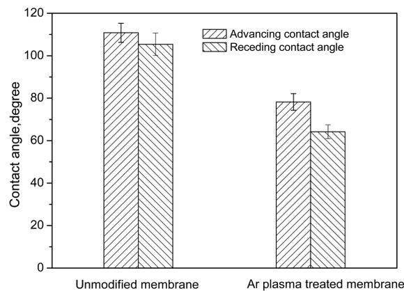
Fig. 2 Advancing and receding water contact angles on the unmodified and modified membrane surface
