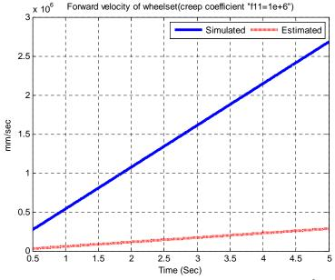
Fig. 3 Forward velocity wheelset at creep co-efficient of 10<sup>6</sup>
