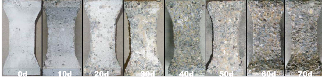
Fig. 2 Surface appearance of concrete specimen exposed to acid solution for various periods
