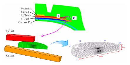
Fig. 3 Crack location (1: center direction, 11: circumferential direction, 21: side direction)
