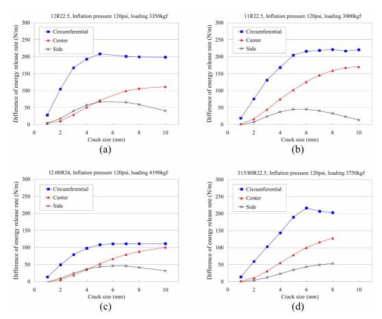
Fig. 6 Difference of energy release rate with respect to the direction of crack propagation: (a) 12R22.5, (b) 11R22.5, (c) 12.00R24, (d) 315/80R22.5 radial truck tires
