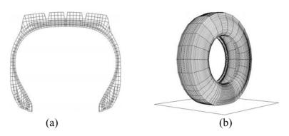
Fig. 2 Global finite element modeling of 12R22.5 tire: (a) 2D model, (b) 3D model
