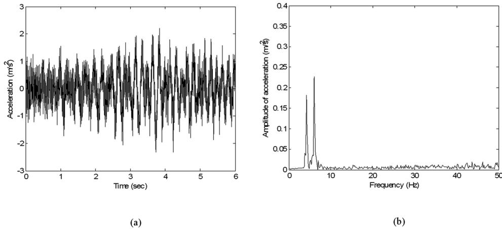
Fig. 9 Responses of test vehicle passing through the bridge with surface roughness ( $v = 5$  m/s): (a) acceleration response, (b) spectrum
