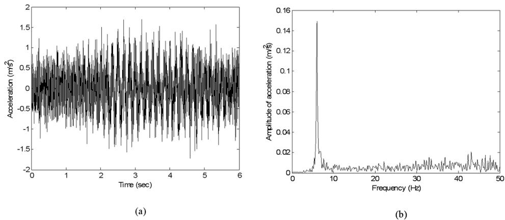
Fig. 8 Responses of single vehicle passing through the bridge with surface roughness: (a) acceleration response, (b) spectrum
