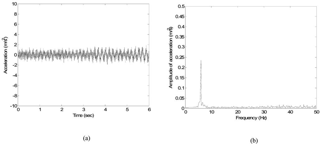
Fig. 5 Responses of vehicle moving on rigid surface with roughness (good condition): (a) acceleration response, (b) spectrum
