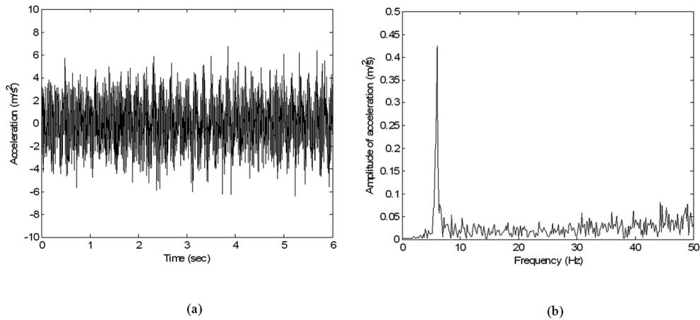
Fig. 7 Responses of vehicle moving on rigid surface with roughness (poor condition): (a) acceleration response, (b) spectrum
