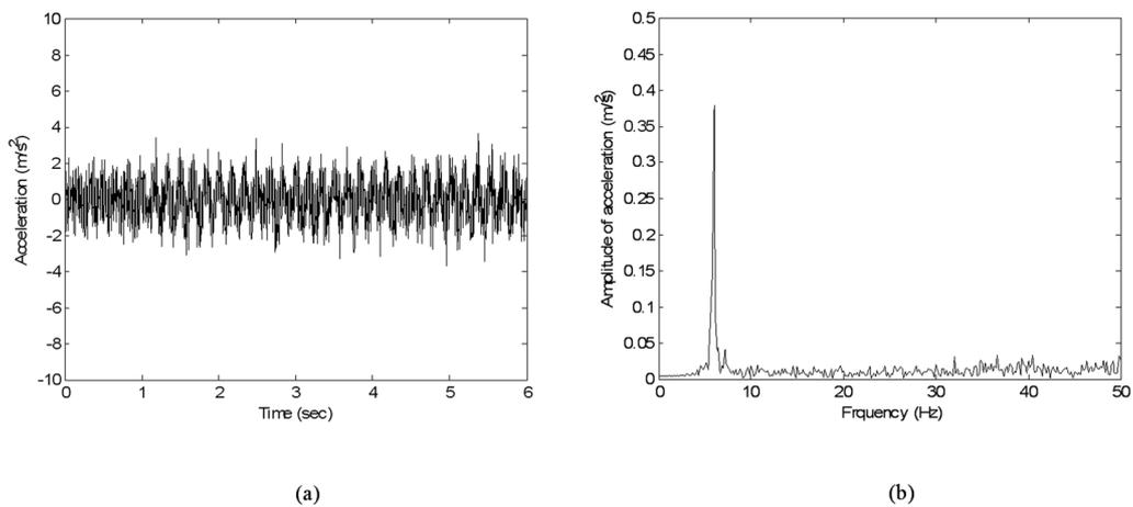
Fig. 6 Responses of vehicle moving on rigid surface with roughness (average condition): (a) acceleration response, (b) spectrum
