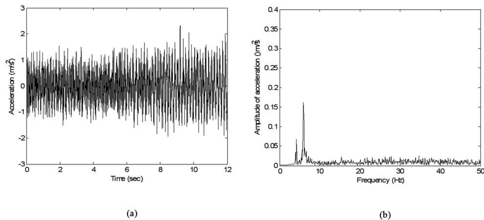
Fig. 11 Responses of test vehicle passing through the bridge with surface roughness ( $v = 2.5$  m/s): (a) acceleration response, (b) spectrum
