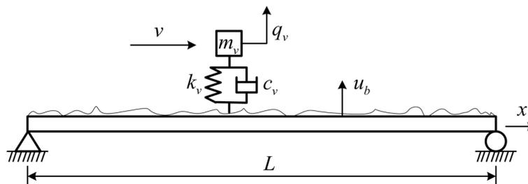
Fig. 1 Mathematical model for vehicle-bridge interaction system
