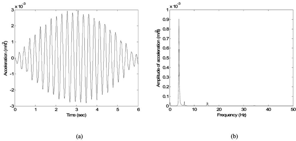
Fig. 4 Responses of vehicle passing through the bridge with smooth surface: (a) acceleration response, (b) spectrum
