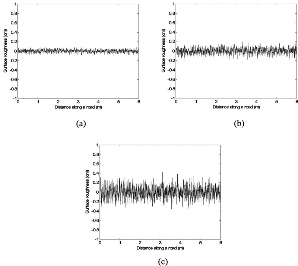
Fig. 3 Profiles of road surface roughness: (a) good, (b) average, (c) poor
