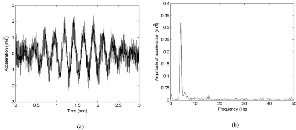
Fig. 10 Responses of test vehicle passing through the bridge with surface roughness ( $v = 10$  m/s): (a) acceleration response, (b) spectrum
